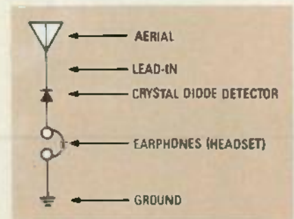
FIG. 1—THE SIMPLEST CRYSTAL RECEIVER consists of an antenna, a detector, headphones, and a ground.
