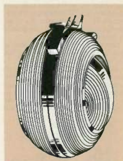
FIG. 8—A VARIO-COUPLER, or variometer, consisted of two coils mounted in such a way that one could be rotated within the other.
